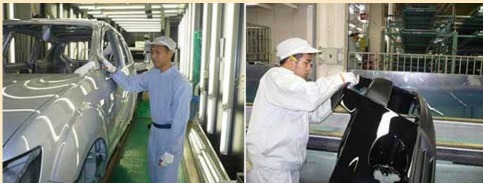
Carefully checking the painted surfaces of vehicles being assembled for foreign particles
