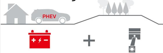
It is possible to use only the electric motor without consuming gasoline for short trips, such as for everyday commuting and shopping. The motor and engine can also be used in combination to extend the driving range, using the engine to generate the electricity when battery levels run low.
