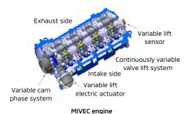
The MIVEC is a variable valve timing mechanism for minimizing fuel consumption. The intake valve lift is continuously varied according to the operating condition to minimize air intake energy loss, resulting in improved fuel efficiency.
