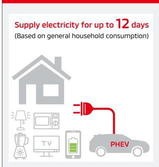
Via a bi directional (V2H\*5) charger, the electricity in the battery and the engine's generating capabilities can be used in combination to supply electricity for up to 12 days\*6. It can also be used as an emergency power source in times of disaster.
