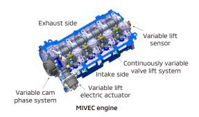
The MIVEC is a variable valve timing mechanism for minimizing fuel consumption. The intake valve lift is continuously varied according to the operating condition to reduce intake resistance. This minimizes air intake energy loss, resulting in improved fuel efficiency.
