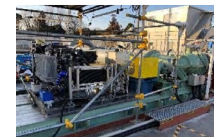
"DELICA D:5" engines driving drainage pumps
