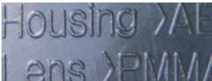
Rear combination lamp markings
