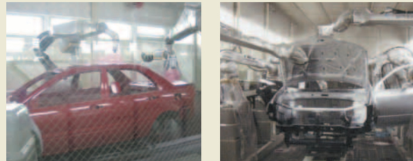
Robots help to reduce the amount of paint used.
