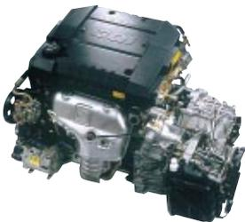
GDI turbo engines take full advantage of the outstanding anti-knocking properties of GDI engines, and at the same time offer better response and fuel efficiency than conventional turbo engines. A GDI turbo engine was adopted for the Pajero io in July 2000, which not only cleared the 2000 exhaust controls, but was also the first turbo car to pass the 2010 fuel efficiency standards.
