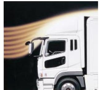
Truck wind tunnel testing
