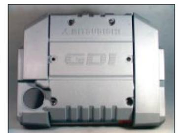
Engine cover made from recycled PET bottles
