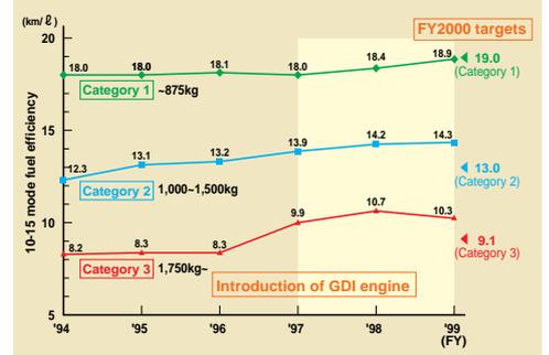
Trends in average fuel efficiency by vehicle weight category (gasoline-powered passenger cars)
