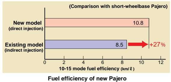
For passenger cars, MMC has developed a new 3.2 l direct injection diesel engine, which was used for the new Pajero model released in September 1999. This new type of engine realizes dramatically improved fuel efficiency combined with increased output due to the optimal design of the high-pressure fuel injection system and combustion chamber and adoption of a DOHC four-valve system.
