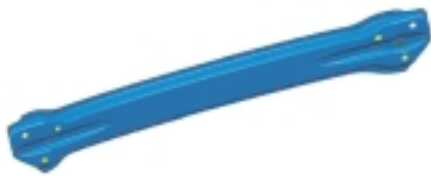
Fig. 2 Hot-stamped bumper beam
