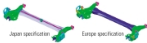
Fig. 7 Torsion axle: Japan specification vs. Europe specification
