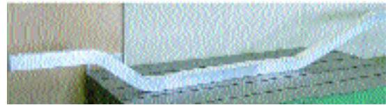
Fig. 4 One-piece side member
